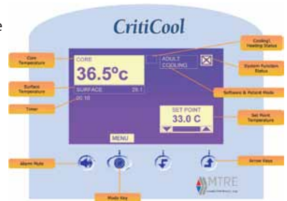
Thermoregulation Control Panel
